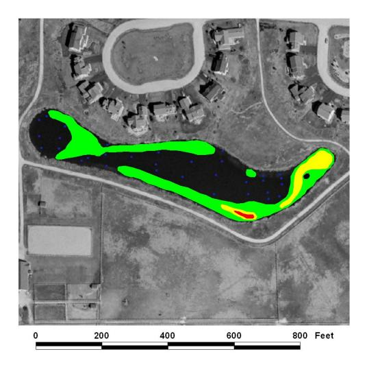
Sediment thickness is based on interpolation between points probed with a 1.5 inch diameter PVC pole graduated in thenths of a foot. Map is based on 59 data points and should be regarded with some margin of error.
